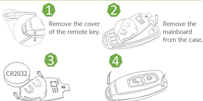
Replace the battery and replace the cover.
