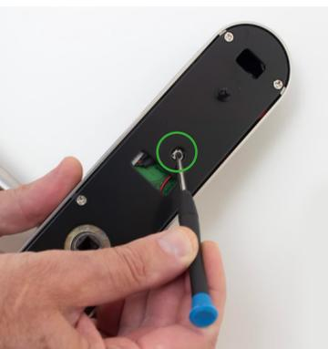
The reset button you can find in the battery compartment of the inner panel. Press the reset button for about 5 seconds until a long sound arises. The handle might ask for an initialisation passcode. This passcode is "0000#". The handle then approves the reset.
