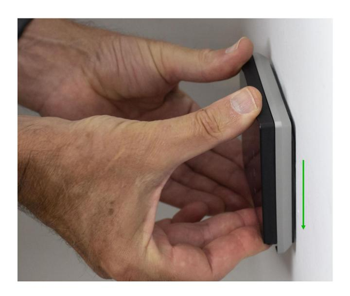
Push the wall reader from top to bottom until it clicks into place on the flush-mounted mounting frame. Then press the locking bar until it clicks into place - CLICK.
