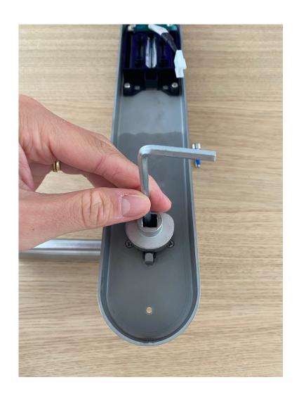
3. After adjusting the direction of the handle, insert it into the handle seat and re-lock the hexagon screw of the handle to the complete the turning.
