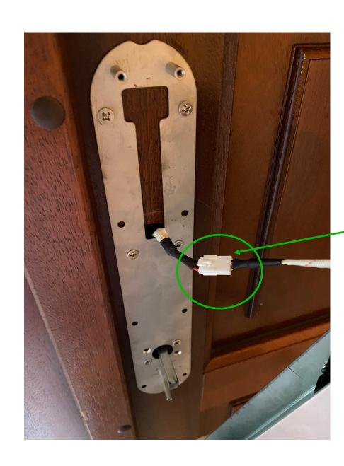
Connect the cable from the front panel with the cable from the back panel.
