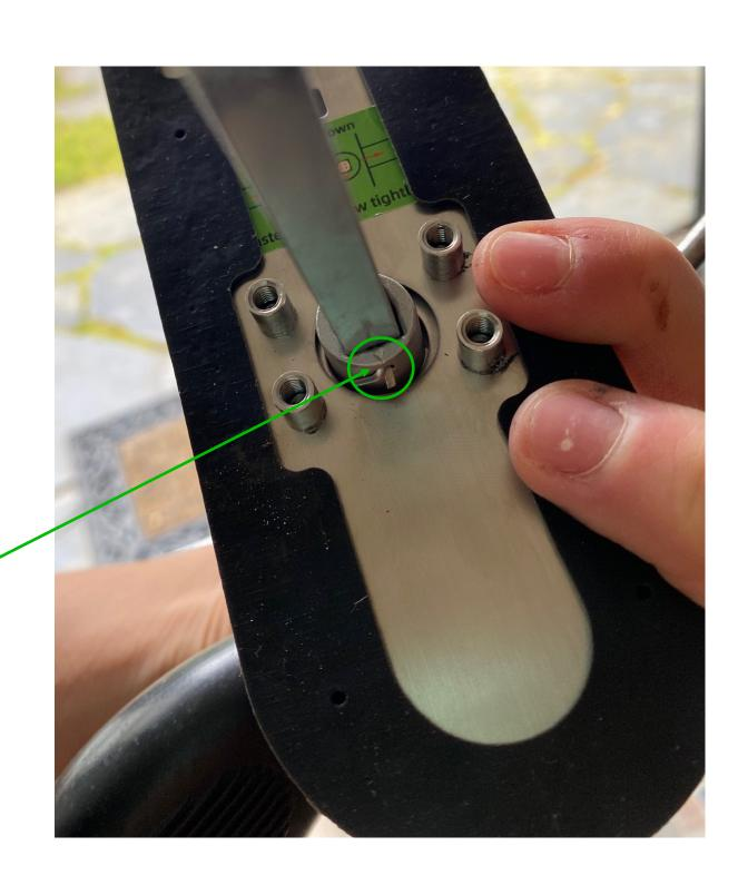
To secure that the motor of the lock is working properly, the arrow always needs to be pointing down when installing!
