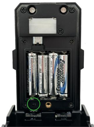
If you do not see the lock in the XL Lock Manager App search list after inserting the batteries, you can do a hard reset of the lock. To do so, press the reset button as shown on the picture for 3 seconds until a long sound arises. After the sound, the lock will be shown in the App, ready to be initialised.
