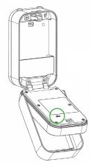
If you do not see the lock in the XL Lock Manager App search list after inserting the batteries, you can do a hard reset of the lock. To do so, press the reset button as shown on the picture for 3 seconds until a long sound arises. After the sound, the lock will be shown in the App, ready to be initialised.
