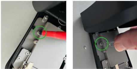
If you do not see the lock in the XL Lock Manager App search list after inserting the batteries, you can do a hard reset of the lock. To do so, press the reset button as shown on the picture for 3 seconds until a long sound arises. After the sound, the lock will be shown in the App, ready to be initialised.
