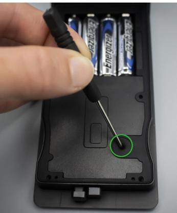
If you do not see the lock in the XL Lock Manager App search list after inserting the batteries, you can do a hard reset of the lock. To do so, press the reset button as shown on the picture for 3 seconds until a long sound arises. After the sound, the lock will be shown in the App, ready to be initialised.
