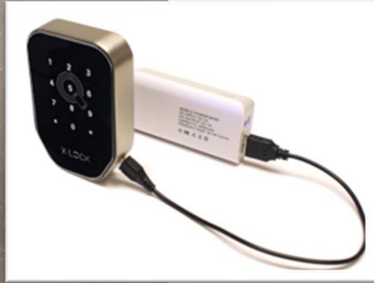
An emergency power supply is possible with any powerbank.
