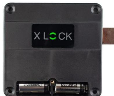
Close the battery compartment cover and fix it with the screw.
